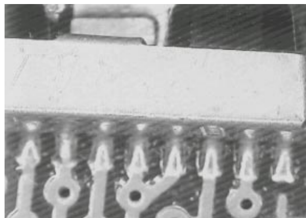
Photo 4.0. Unit self-aligns after reflow.
