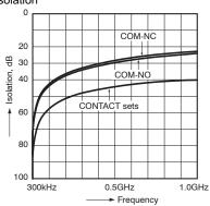
1-(2). High frequency characteristics (Impedance 75 $\Omega$
