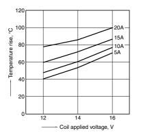
1.-(2) Coil temperature rise (85°C 185°F) Sample: CP1-12V, 6pcs Point measured: Inside the coil Contact carrying current, 5A, 10A, 15A, 20A Resistance method, ambient temperature 85°C 185°F
