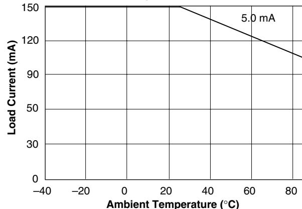
Both relays on with equal load currents.
