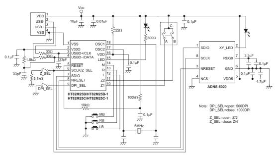
Note: Place the  $0.1\mu\text{F}$  capacitor,  $22\Omega$  resistor and  $0.01\mu\text{F}$  capacitor as close to VDD pin as possible.
