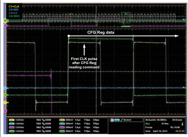
Figure 14. Configuration register reading sequence (zoom)
