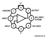
Note: Pin 4 connected to case
