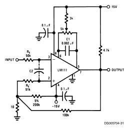
FIGURE 3. Positive Feedback with High Source Resistance
