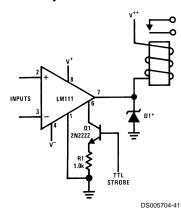
\*Absorbs inductive kickback of relay and protects IC from severe voltage transients on  $\mathsf{V}^{++}$  line.
