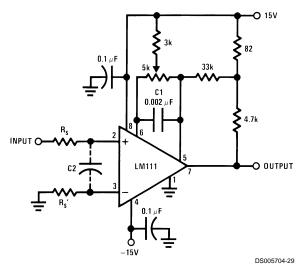
Pin connections shown are for LM111H in the H08 hermetic package
