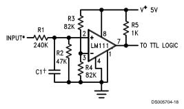
$<sup>^{\</sup>star}\mbox{Values}$  shown are for a 0 to 30V logic swing and a 15V threshold.
