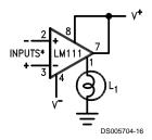
\*Input polarity is reversed when using pin 1 as output.
