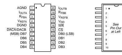
20 Pin CDIP, PDIP (0.300") D20, N20 20 Pin SOIC (Jedec, 0.300") S20
