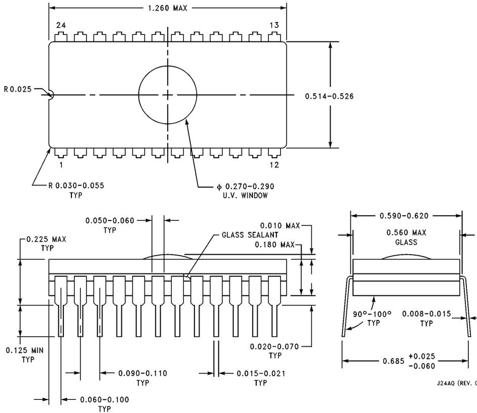
**UV Window Cavity Dual-In-Line Cerdip Package (JQ)**
