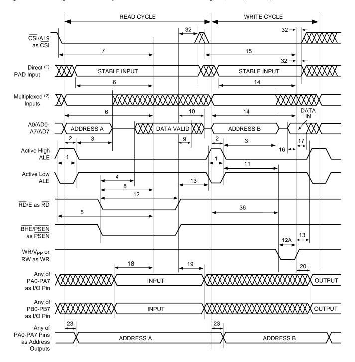
Figure 21. Timing of 8-Bit Multiplexed Address/Data Bus Using RD, WR (PSD3X2/3X3)
