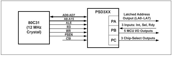
16.0 Power Management (cont.) All the inputs shown, except  $\overline{CSI}$ , go to the PAD logic. These signals must be taken into consideration when calculating the composite frequency. Before we make the calculation, let's establish the following conditions:
