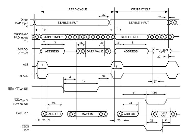
Figure 39. Port A as ADO-AD7 Timing (Track Mode) Using  $R/\overline{W}$ , E or  $R/\overline{W}$ ,  $\overline{DS}$  (PSD3X1)
