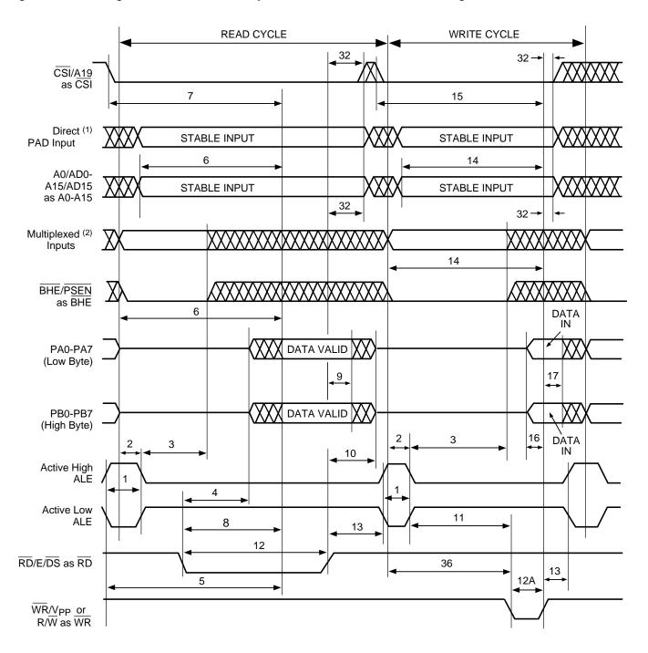
Figure 34. Timing of 16-Bit Non-Multiplexed Address/Data Bus Using  $R/\overline{W}$ , E or  $R/\overline{W}$ ,  $\overline{DS}$  (PSD3X1)
