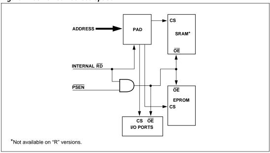
Figure 10. 8031-Compatible Separate Code and Data Address Spaces
