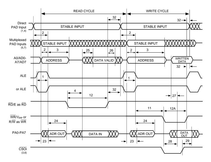
Figure 38. Port A as AD0-AD7 Timing (Track Mode) Using  $\overline{RD}$ ,  $\overline{WR}$  (PSD3X2/3X3)
