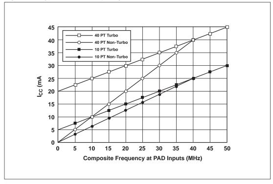
Figure 15. Typical  $I_{CC}$  vs. Frequency ( $V_{CC} = 3 V$ )
