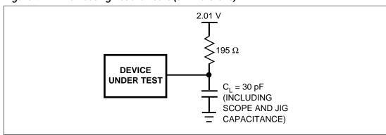
Figure 42B. AC Testing Load Circuit (3 V Versions)
