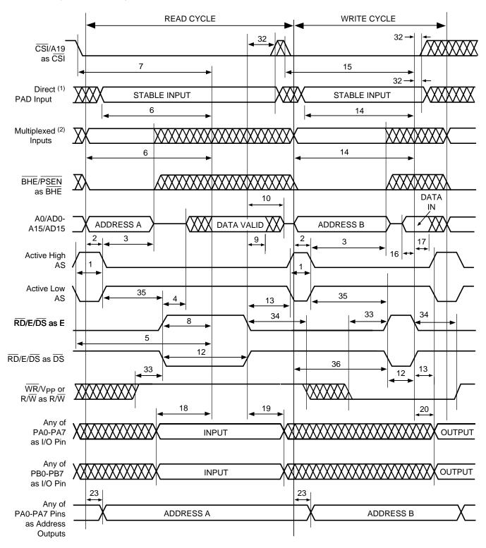
Figure 28. Timing of 8-Bit Non-Multiplexed Address/Data Bus Using RD, WR (PSD3X1)
