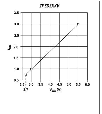
Figure 18. Normalized  $I_{CC}$  (AC) ( $V_{CC} = 3.0 \text{ V}$ )
