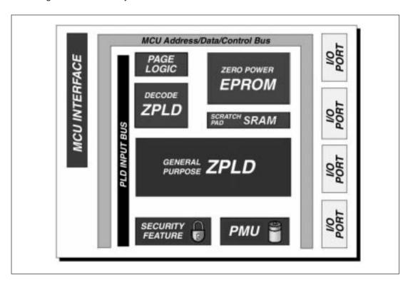
The PSD3XX family architecture (Figure 1) can efficiently interface with, and enhance, almost any 8- or 16-bit microcontroller system. This solution provides microcontrollers the following:
