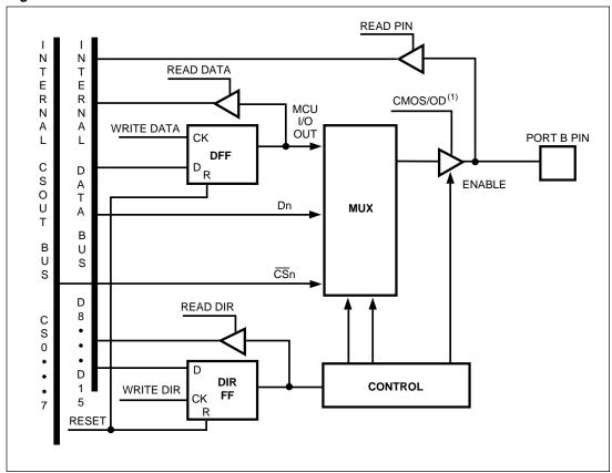
NOTE: 1. CMOS/OD determines whether the output is open drain or CMOS.
