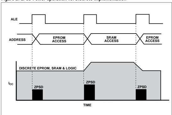
Figure 2. ZPSD Power Operation vs. Discrete Implementation
