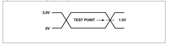
Figure 41B. AC Testing Input/Output Waveform (3 V Versions)
