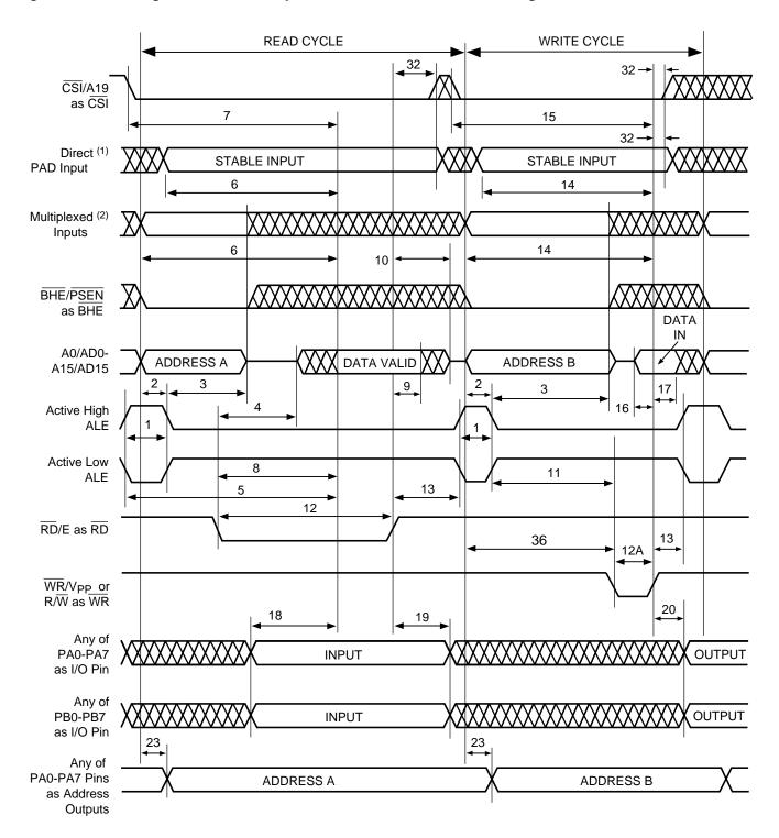
Figure 25. Timing of 16-Bit Multiplexed Address/Data Bus Using RD, WR (PSD3X2/3X3)
