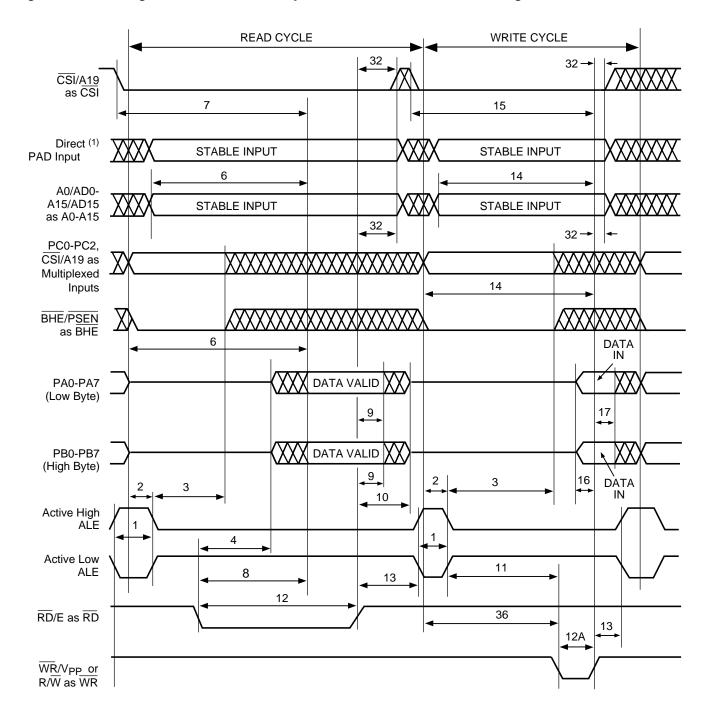
Figure 33. Timing of 16-Bit Non-Multiplexed Address/Data Bus Using RD, WR (PSD3X2/3X3)
