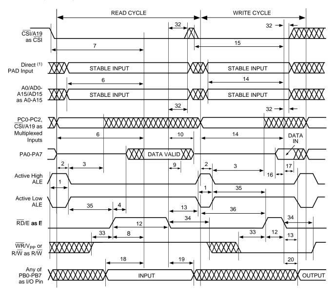
Figure 31. Timing of 8-Bit Non-Multiplexed Address/Data Bus Using  $R/\overline{W}$ , E or  $R/\overline{W}$ ,  $\overline{DS}$  (PSD3X2/3X3)
