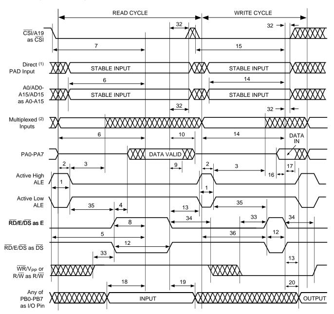
Figure 32. Timing of 16-Bit Non-Multiplexed Address/Data Bus Using RD, WR (PSD3X1)
