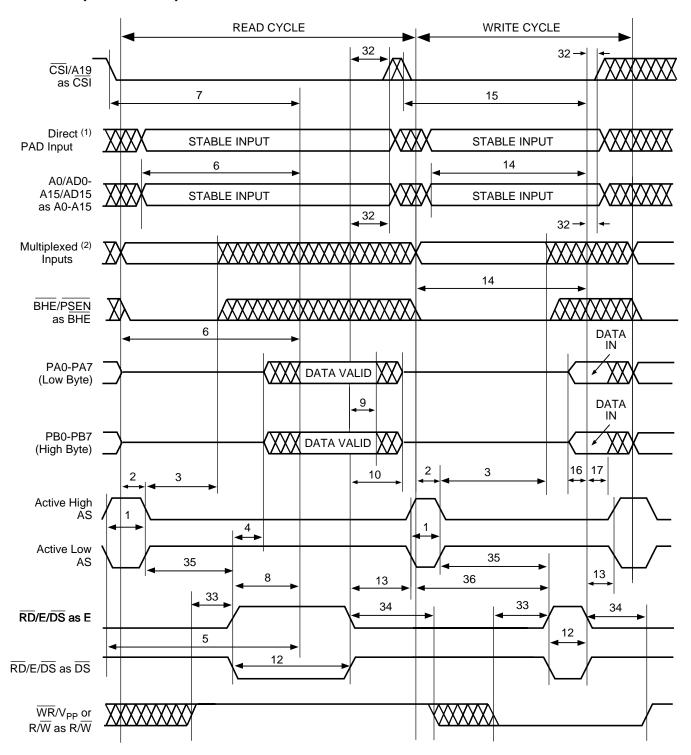
Figure 36. Chip-Select Output Timing
