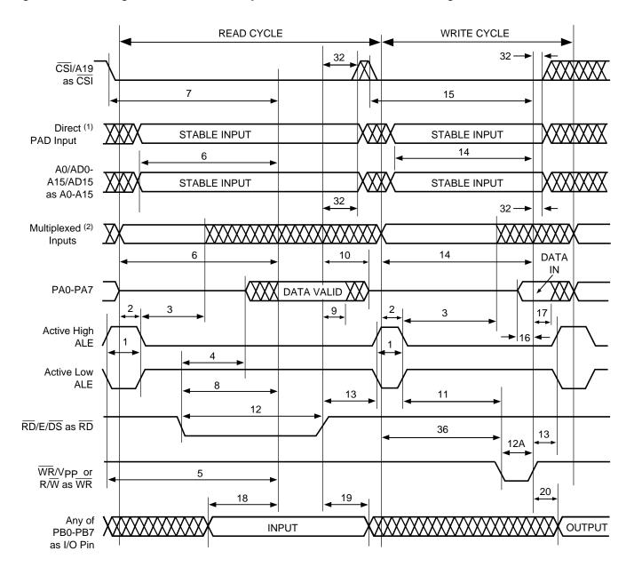
Figure 30. Timing of 8-Bit Non-Multiplexed Address/Data Bus Using  $R/\overline{W}$ , E or  $R/\overline{W}$ ,  $\overline{DS}$  (PSD3X1)
