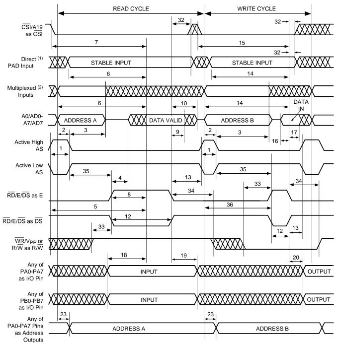
Figure 24. Timing of 16-Bit Multiplexed Address/Data Bus Using RD, WR (PSD3X1)
