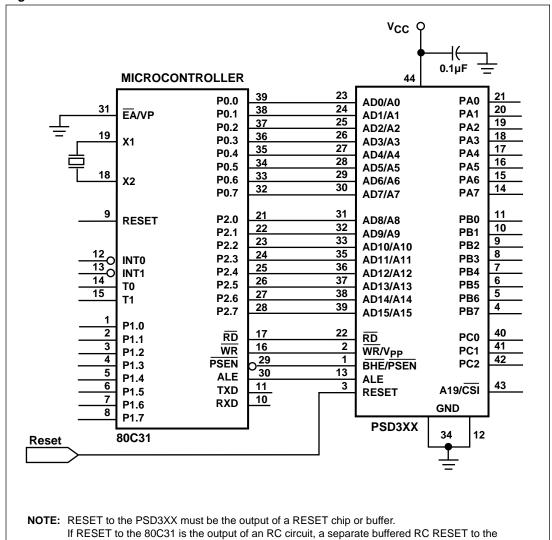
PSD3XX (shorter than the 80C31 RC RESET) must be provided to avoid a race condition.
