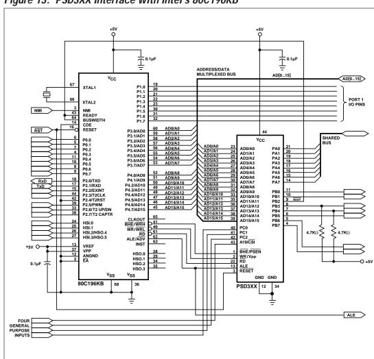
Figure 13. PSD3XX Interface With Intel's 80C196KB
