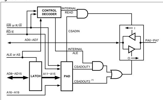
NOTE: 1. The expression for CSADOUT2 must include the following write operation cycle signals: For CRRWR = 0, CSADOUT2 must include WR = 0.
