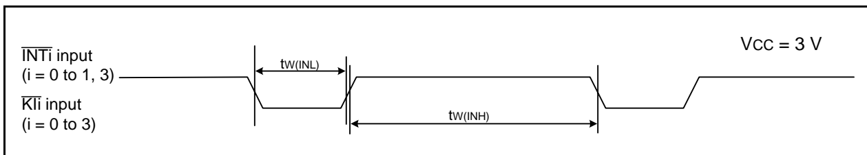
Figure 5.14 Input Timing Diagram for External Interrupt \overline{INTi} and Key Input Interrupt \overline{Kli} when Vcc = 3 V
