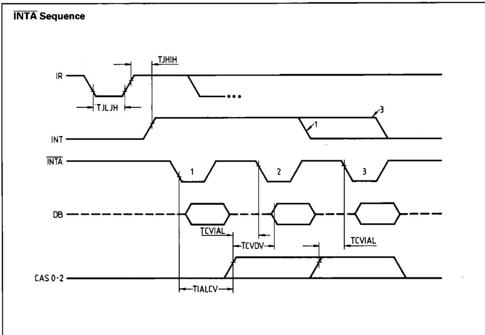
**Notes:** Interrupt output must remain high at least until leading edge of first  $\overline{INTA}$ .
