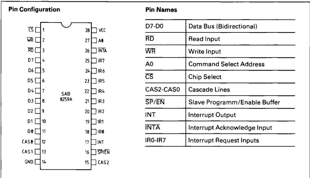
The SAB 8259A programmable interrupt controller handles up to eight vectored priority interrupts for the CPU. It is cascadable for up to 64 vectored priority interrupts without requiring additional circuitry. The SAB 8259A is fabricated in +5V advanced N-channel, silicon gate Siemens MYMOS technology and packaged in a 28-pin DIP. The circuitry is static, requiring no clock input.
