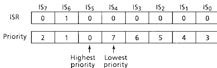
Figure 4.6 The Example of Interrupt Priority Transition in Automatic Rotation Mode
