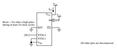
Figure 16.  $I_{CC}$  Test Condition, Power-Down Mode
