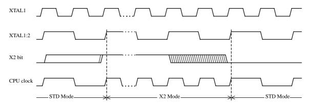
Figure 2. Mode Switching Waveforms
