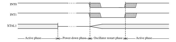
Figure 10. Power-Down Exit Waveform
