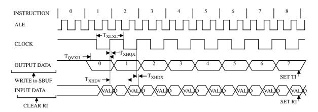
Figure 21. Shift Register Timing Waveforms
