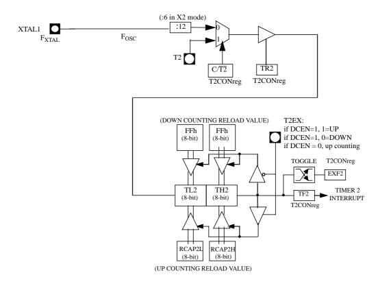
Figure 4. Auto-Reload Mode Up/Down Counter (DCEN = 1)
