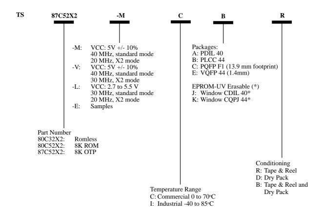
(\*) Check with Atmel Wireless & Microcontrollers Sales Office for availability. Ceramic packages (J, K) are available for prototyping, not for volume production.
