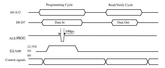
Figure 12. Programming and Verification Signal's Waveform
