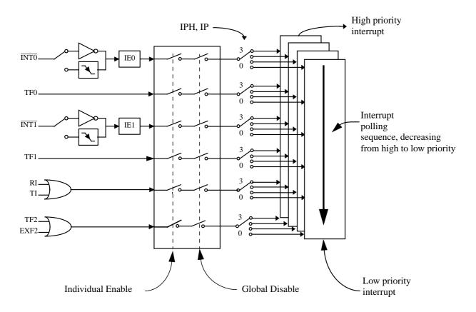
Figure 9. Interrupt Control System
