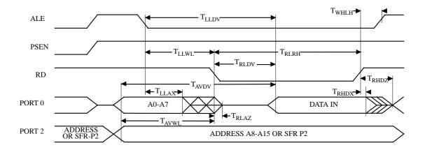
Figure 20. External Data Memory Read Cycle
