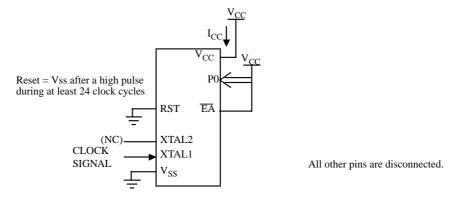
Figure 14. Operating  $I_{CC}$  Test Condition
