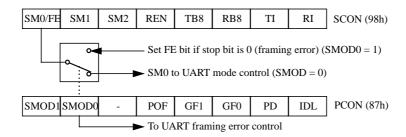
Figure 6. Framing Error Block Diagram
