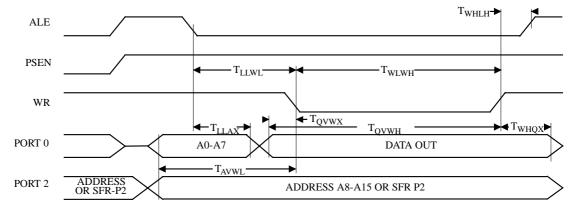
Figure 19. External Data Memory Write Cycle
