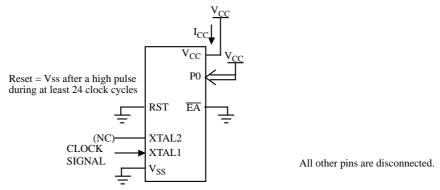
Figure 15.  $I_{CC}$  Test Condition, Idle Mode
