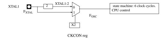
Figure 1. Clock Generation Diagram
