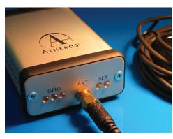
Complete with software and an integrated uN3010 daughterboard, the ORION RX2 Evaluation Kit (EVK) is a full-featured GPS receiver that provides a conventional platform to evaluate the performance of the ORION RX2 $^{\text{M}}$ .
