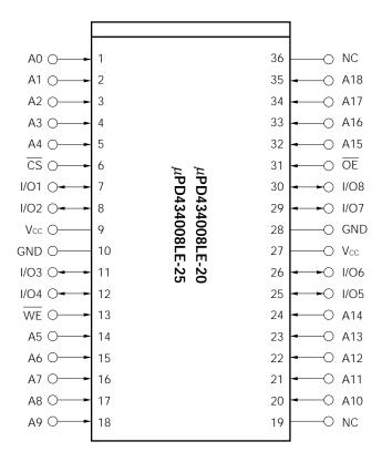
A0 – A18 : Address inputs I/O1 – I/O8 : Data inputs/outputs
