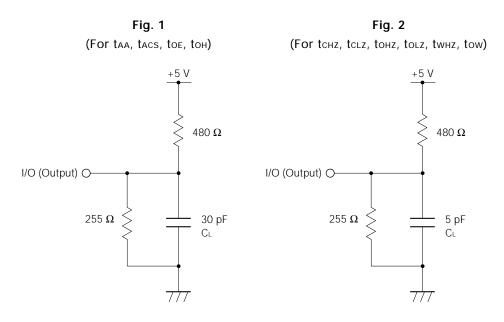
**Remark** C<sub>L</sub> includes capacitances of the probe and jig, and stray capacitances.
