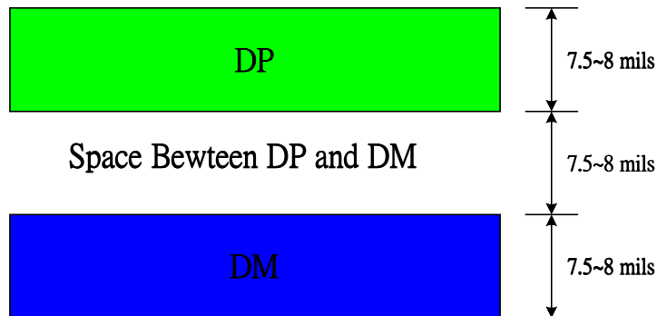
Figure 11. USB Differential Signal Routing
