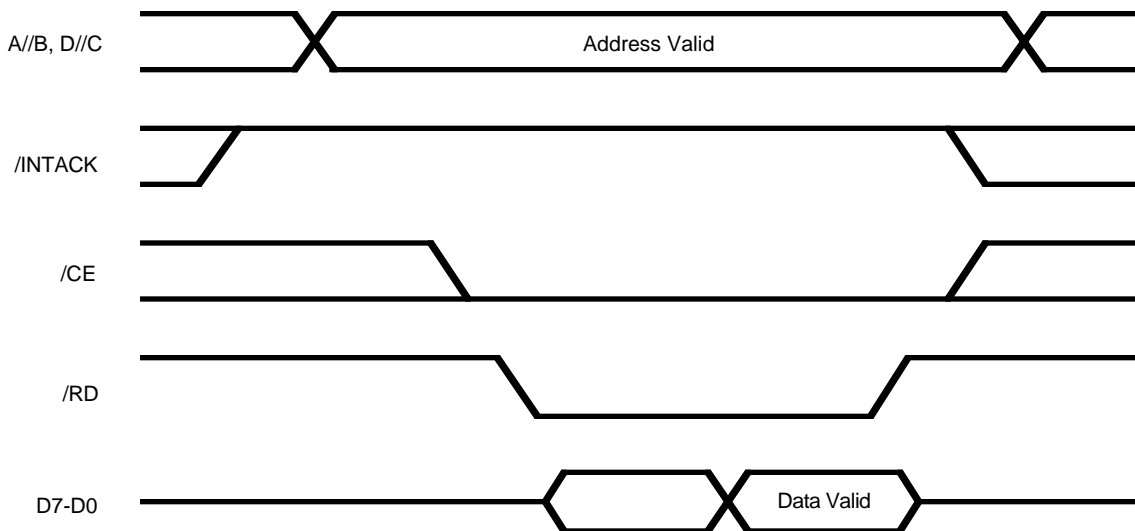
Figure 2-5. Z85X30 Read Cycle Timing
